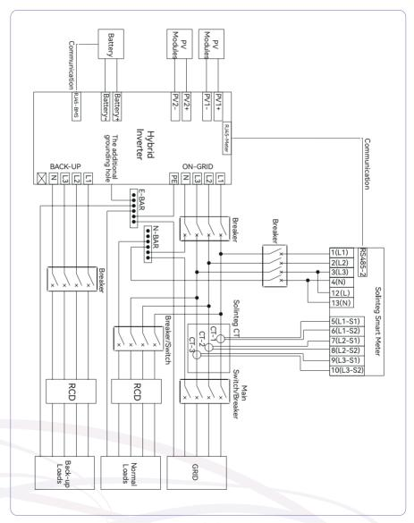
Figure 5-2 Standard wiring diagram
