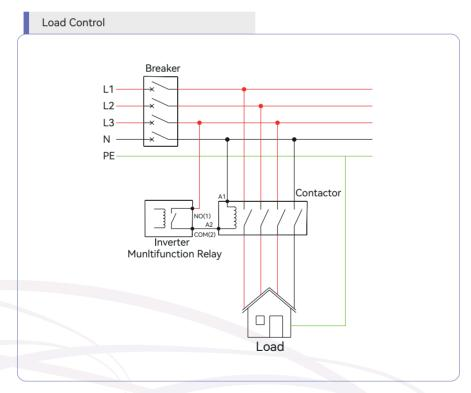
Figure 5-25 Load control connection diagram
