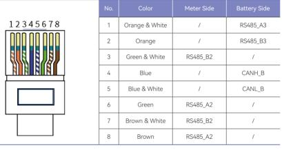
Figure 5-24 RJ45 terminal connection sequence and definition
