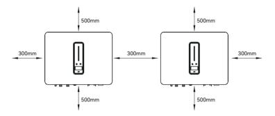
Figure 4-2 Recommended installation spacing
