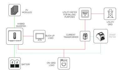
Figure 3-1 Schematic diagram of hybrid system
