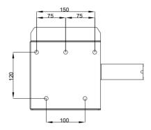
Figure 4-4 Dimensions of wall bracket
