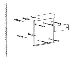
Figure 4-6 Fixing the wall bracket
