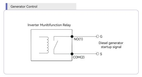
Figure 5-26 Generator Control connection diagram
