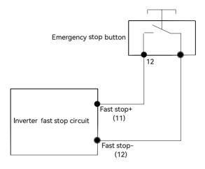
Figure 5-28 Fast stop connection diagram
