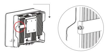
Figure 4-7 Mounting the inverter
